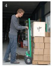
Ensure that the load on the workbench which is to be lifted down does not exceed the weight limit of 75 kilograms. If the load exceeds this weight, a hazardous situation may occur which should be prevented at all times.
